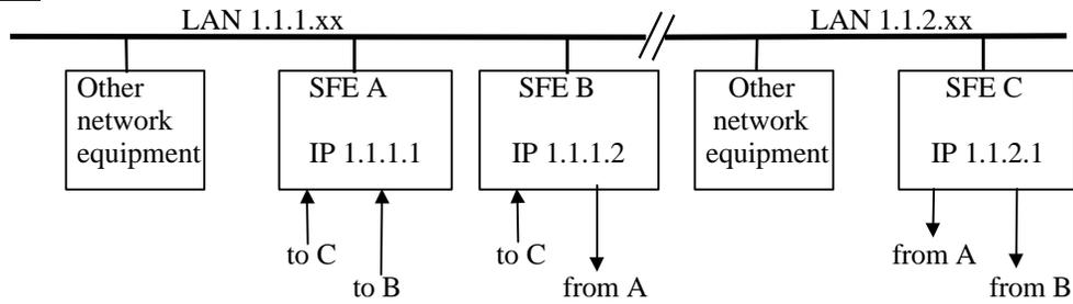
SFE allows you to make and break connections between units, examine and change configurations, unit names, IP numbers etc. of any SFE on the network. Security is provided by a password for each unit.
