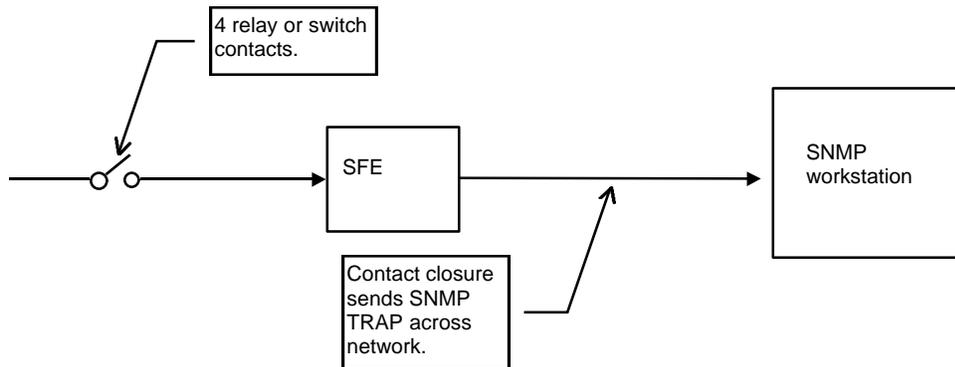
Using SNMP, the outputs can be set or reset. E.g. reset or power cycle a remote system -
