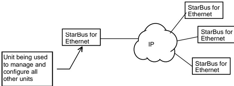
SFE provides error corrected, self repairing logical links. Every network packet is error checked and sequence numbered to ensure all your data is delivered and is error free. Should the network or the power fail, the SFEs will automatically re-link when the problem is resolved. To keep network loading to a minimum, SFE only passes packets to the network when there is data to be forwarded.
